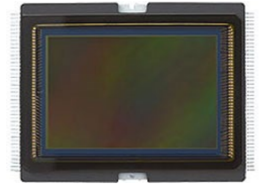
Canon 6D sensor (20.20 MP, full-frame)
