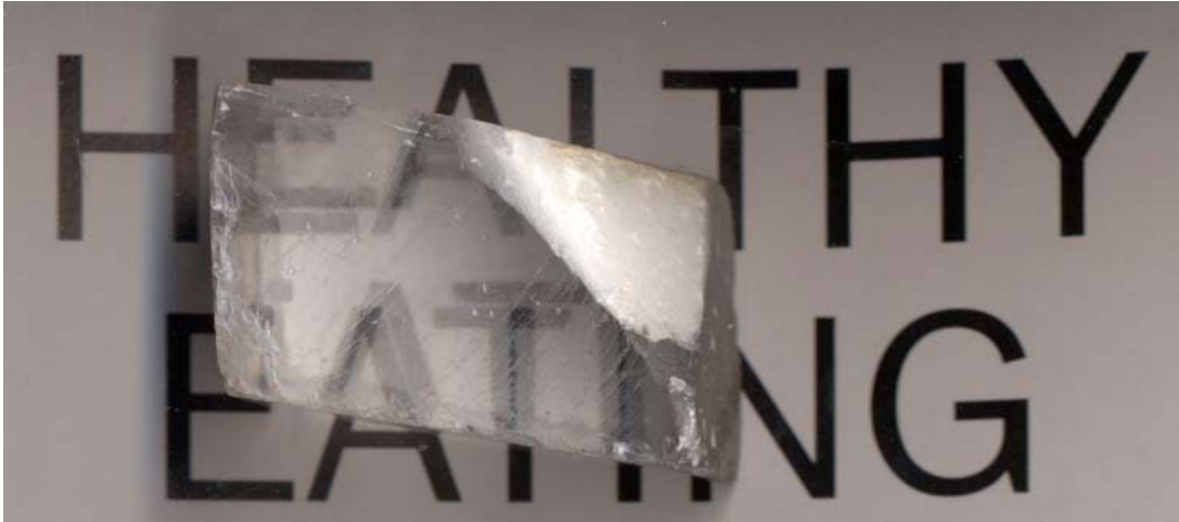
birefringence in a calcite crystal
