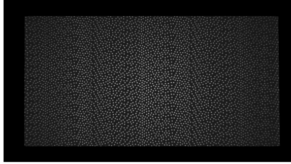
Figure D. Calibrated projector pattern for Intel RealSense D435.
