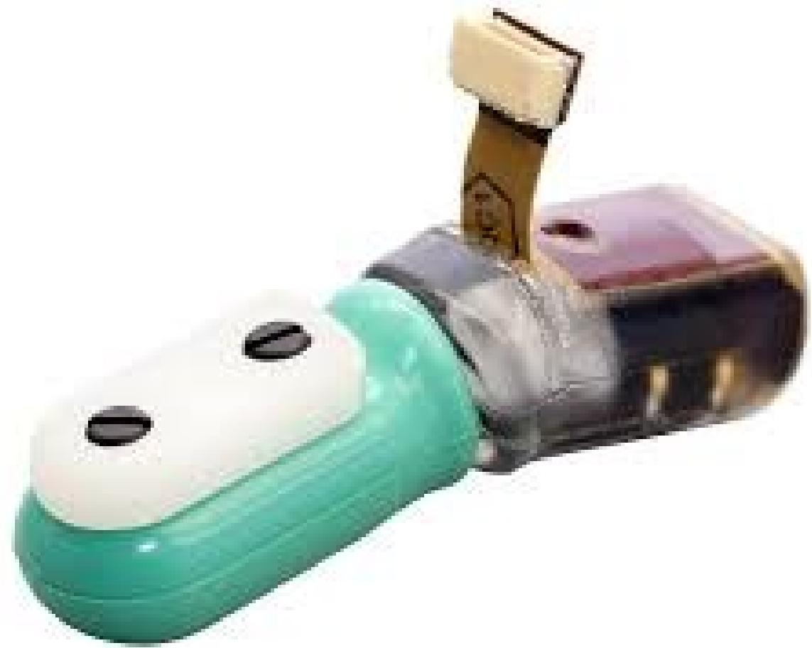
BioTac ionically-conductive fluid based
