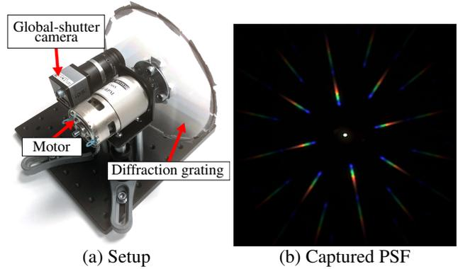
Figure 6. Image of our hardware setup, consisting of a global-shutter camera and a circular diffraction grating attached to a 20,000 RPM motor.
