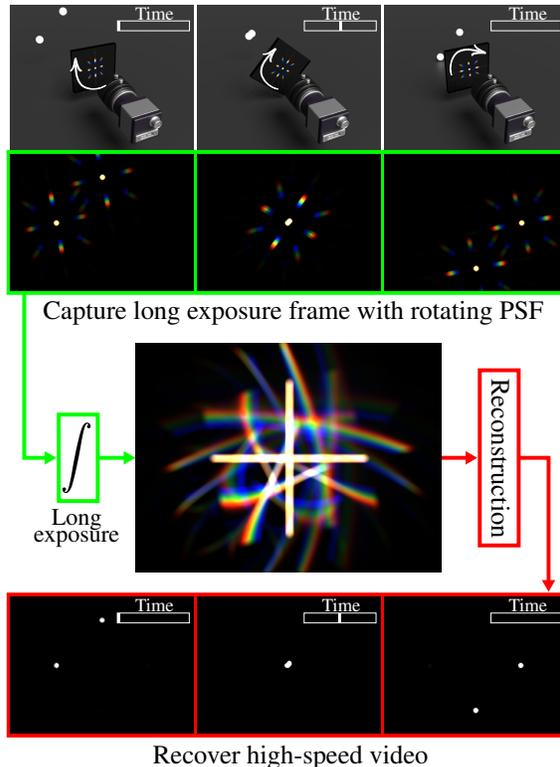
Figure 1. **Principle of high-speed imaging with a rotating diffraction grating.** A camera captures a long exposure image of a moving scene. During the camera’s exposure period, the diffraction grating placed in front of the camera continuously rotates to generate a time-varying point-spread function (PSF) that encodes scene dynamics into a single frame. Solving a deconvolution problem yields a high-speed video from the captured frame.
