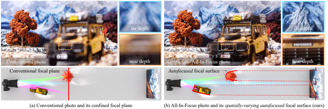
Figure 1. Spatially-varying autofocus to produce an optical all-in-focus image. Left: A conventional photo with a regular lens, where objects at a single focal plane appear sharp. Right: An all-in-focus photo captured through spatially-varying autofocusing. To achieve this, we combine (i) a programmable lens with spatially-varying control over focus, and (ii) a spatially-varying autofocus algorithm to drive the focus of this lens. Note that this is an optically-captured image of a real scene with no post-capture processing used.
