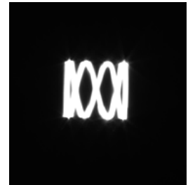
Figure 7. Lissajous curve scanned in the focal plane of the collimating lens.
